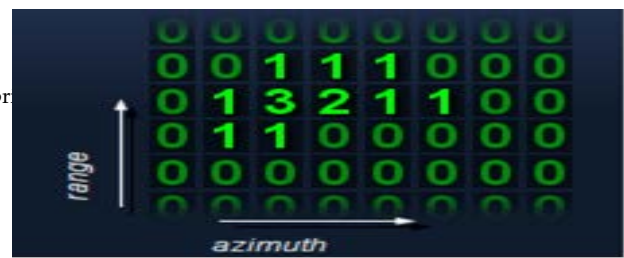
Figure 7: The Signal Processor provides hits including information about received power
